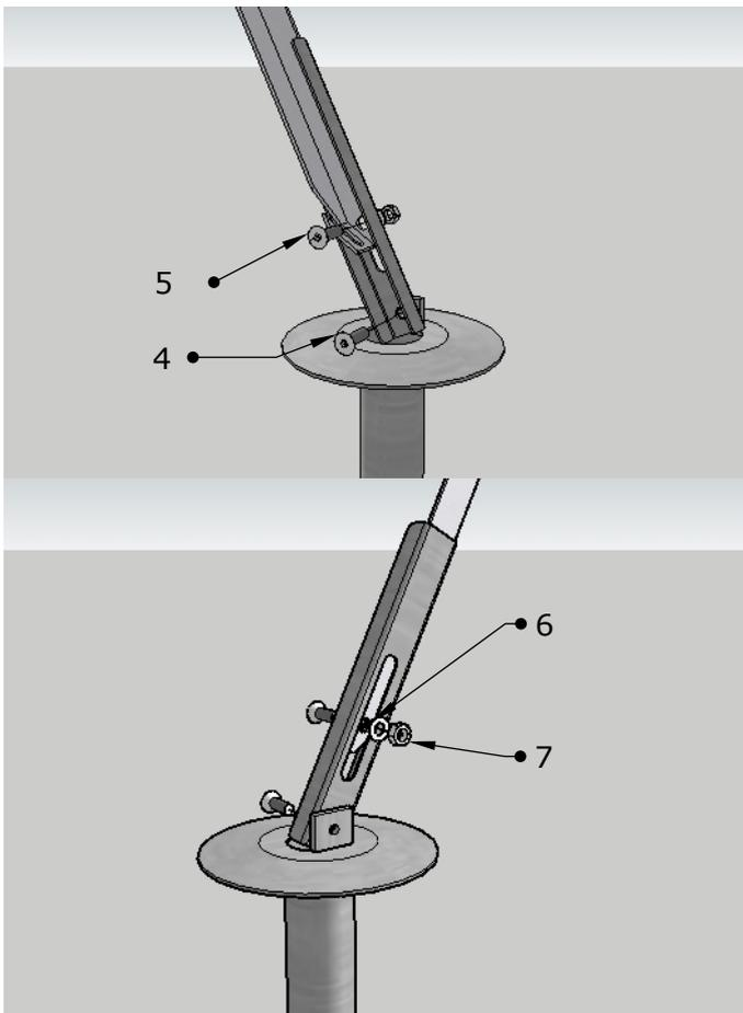
FISSARE LA SAETTA E LA STAFFA PER SAETTA COME RIPIORTATO IN FIGURA 4 CON:
